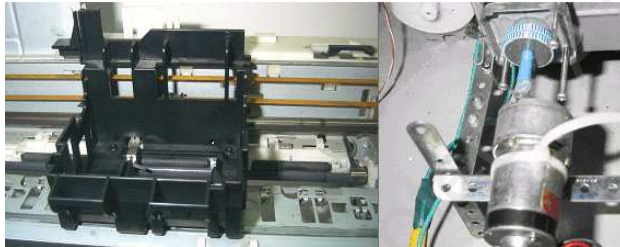
Fig. 5. Drive components: (left) rail and toothed belt, (right) actuator (DC motor coupled with gear train).
