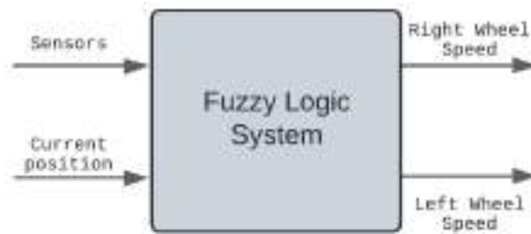
Figure 2.14: Black Box Diagram of Fuzzy Logic System Implementation
