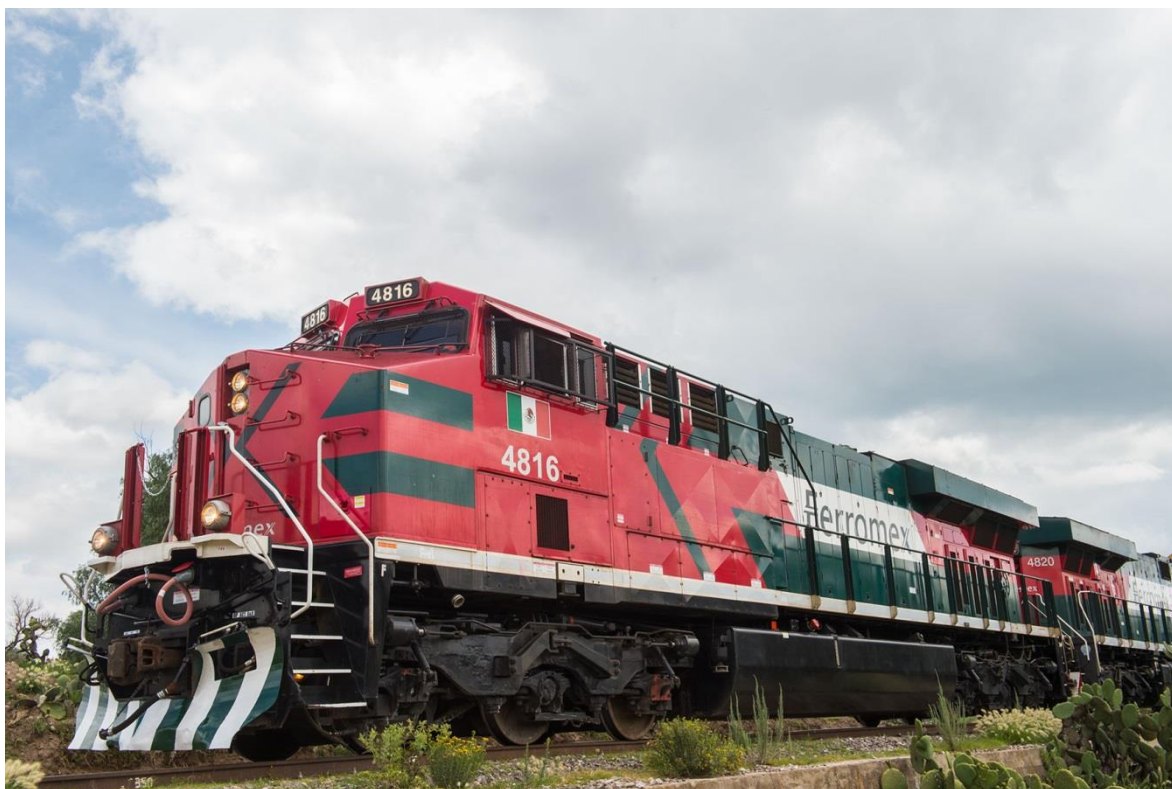
Figura 5 - Máquina FFE-4816 (Modelo G.E. ES-4,400AC, 2016, 6 ejes, AC, 4,400 HP's)
