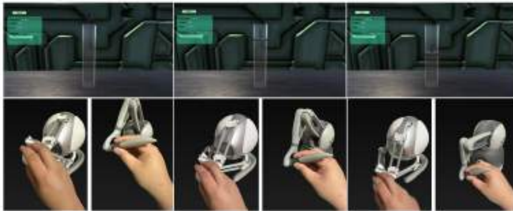
Figure 2. Visuo-haptic simulator interaction process illustrating piston displacement and corresponding hand movement on the haptic device. As the piston is displaced, the simulator calculates the corresponding pressure values and displays them in real time, while also delivering proportional resistance through the haptic device. This combination of visual and tactile feedback highlights the inverse relationship between pressure and volume.
